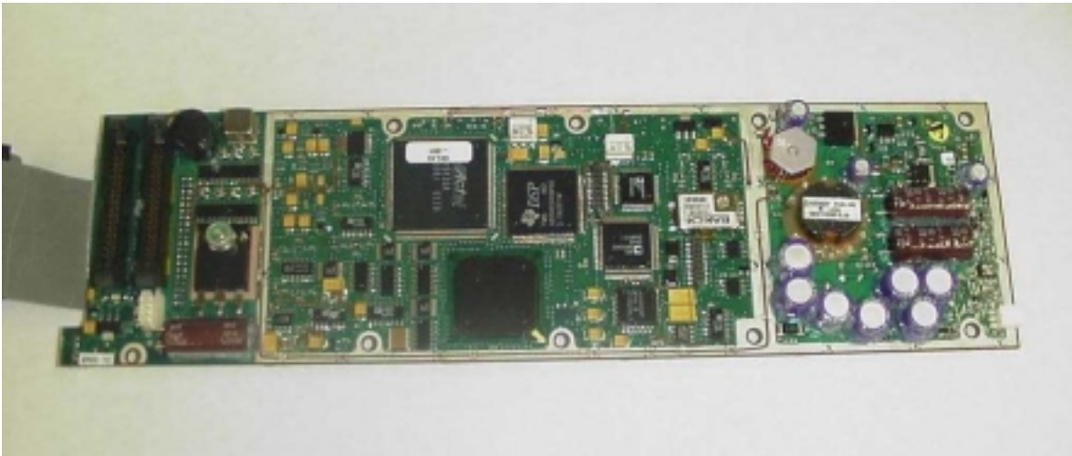
Photo 1: DSP/Power Supply Circuit Card, Top View
