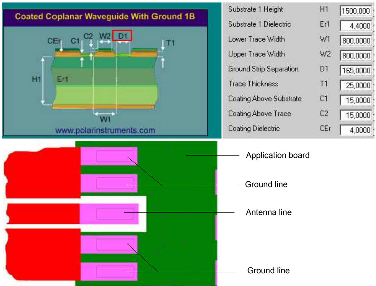
Figure 15: Micro-Stripline on 1.5mm Standard FR4 PCB - example 1
