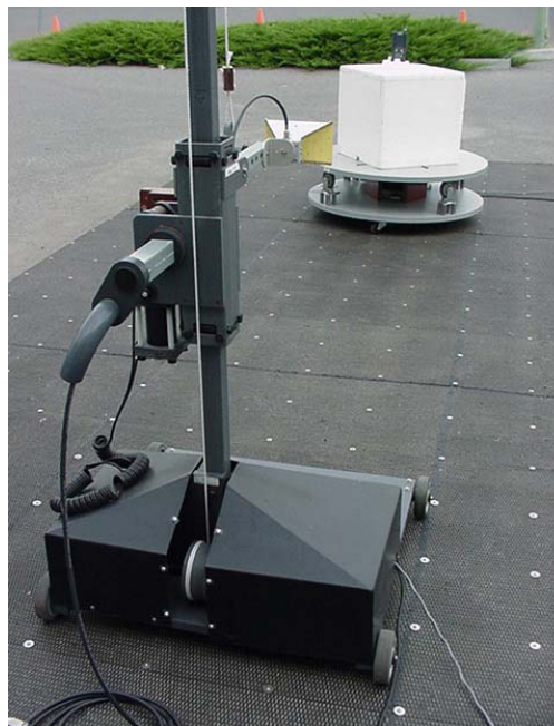
Photograph C.7-3 - Dipole Substitution Antenna Setup
