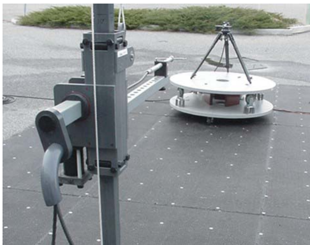
Photograph C.7-3 - Dipole Substitution Antenna Setup
