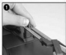
push the arm lock to release the tone-arm.
