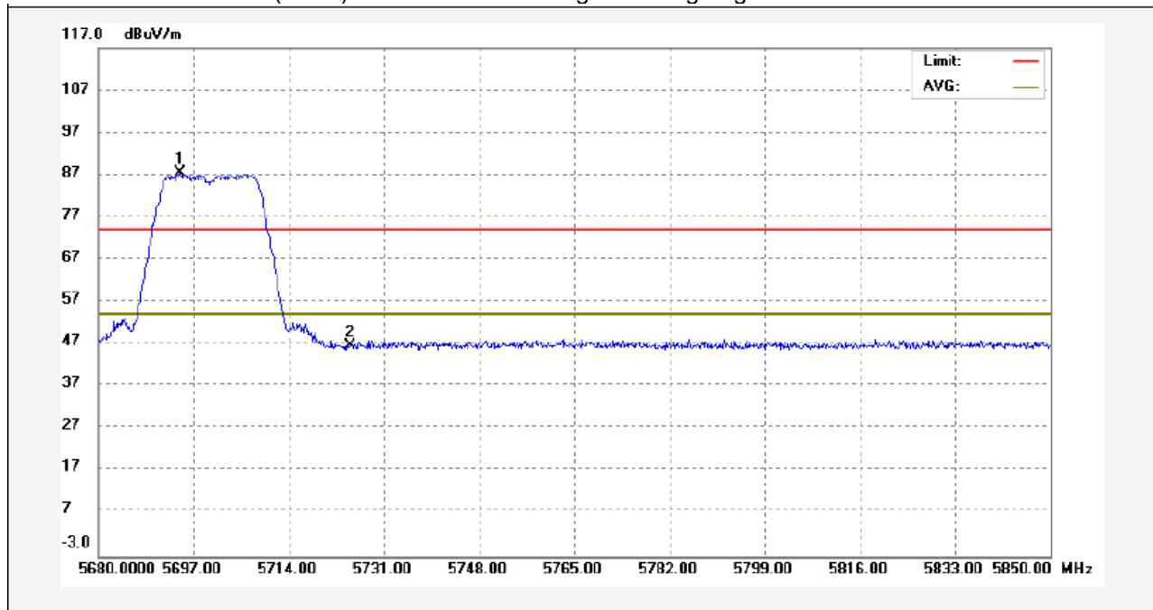
802.11ac(HT20) U-NII-2C Transmitting Band edge-right side Horizontal
