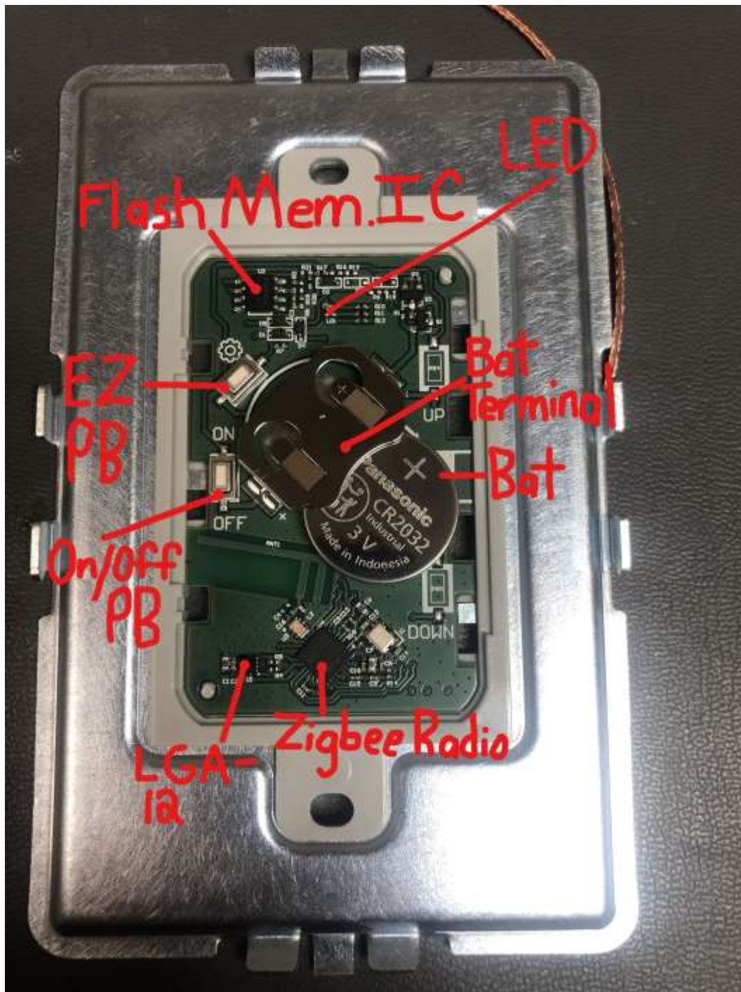
Internal Photo Legrand Model WNAL23 PCB View With Zigbee Radio Location
