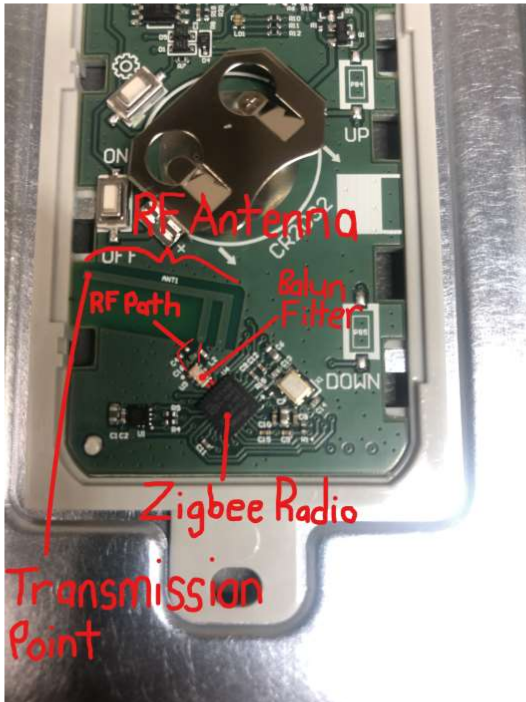
Internal Photo Legrand Model WNAL23 PCB View With Zigbee Radio Antenna Location
