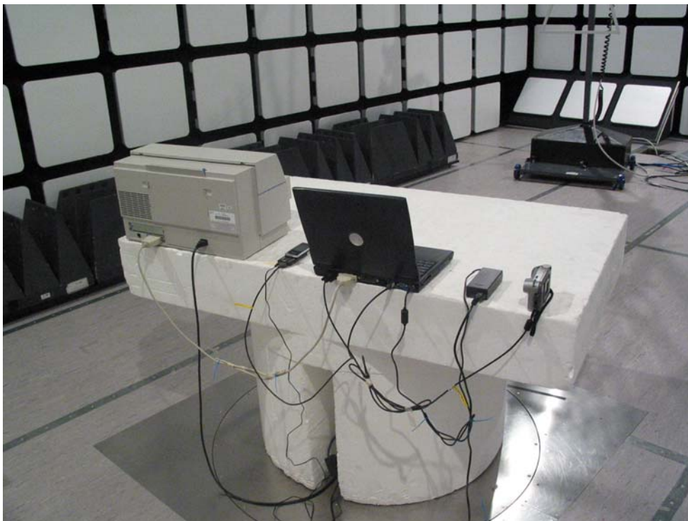
Picture 2 Radiated emission measurement
