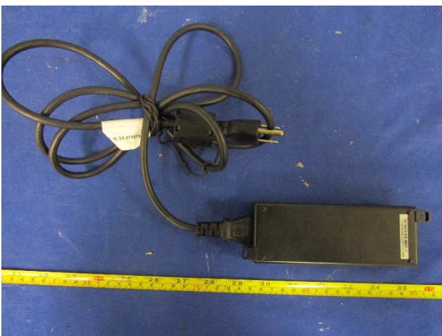
Support Equipment Power Supply Top View
