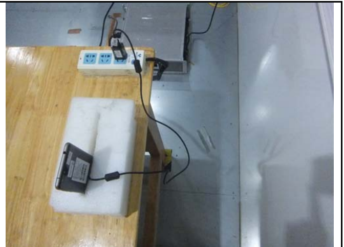
Conducted Emissions Test Setup Side View
