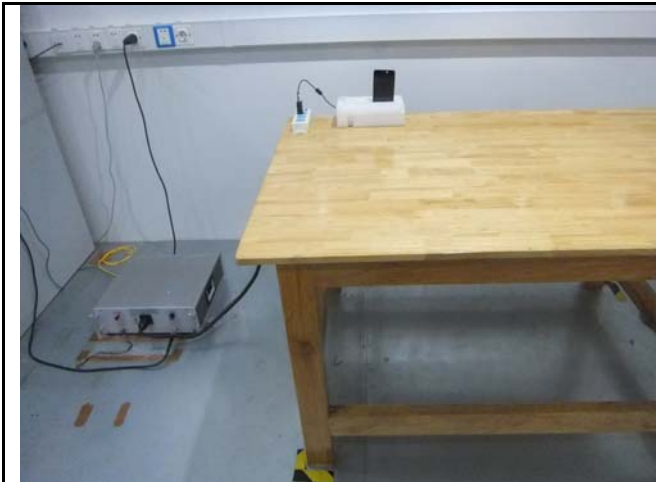
Conducted Emissions Test Setup Front View
