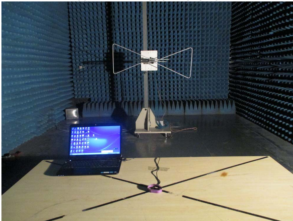
FCC RADIATED EMISSION TEST SETUP
