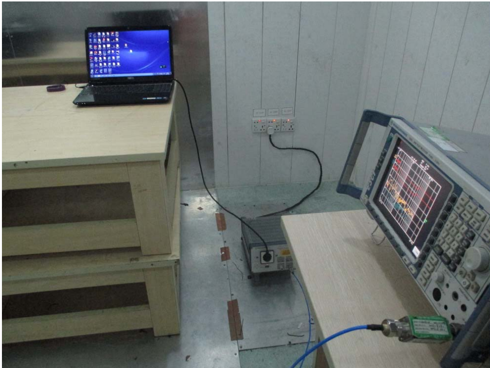
FCC RADIATED EMISSION TEST SETUP
