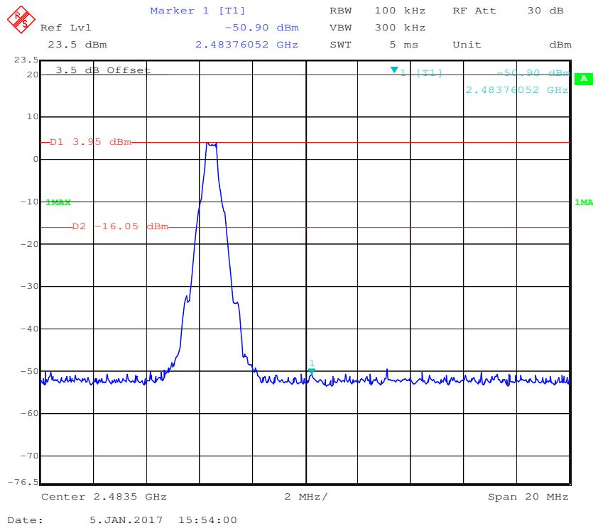
**EDR ( $\pi/4$ -DQPSK): Band Edge-Left Side**
