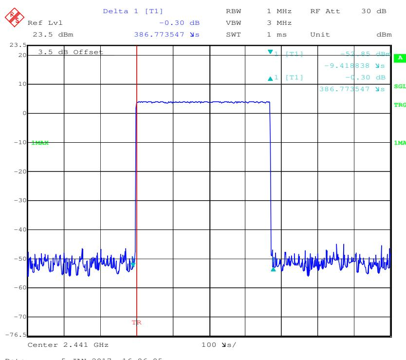
**Pulse time, High Channel, DH1**
