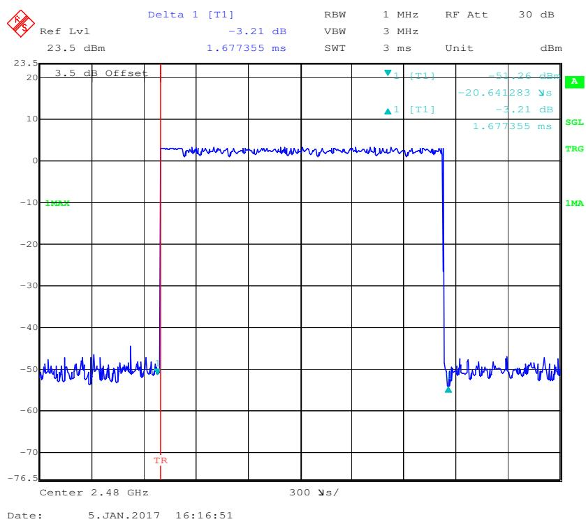
**Pulse time, Low Channel, 3DH5**
