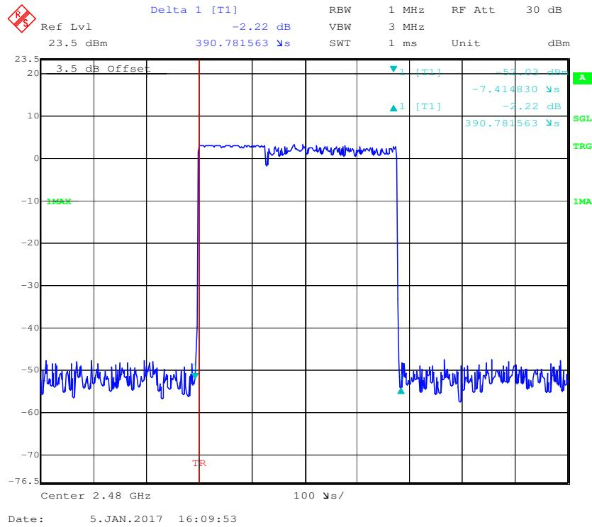
**Pulse time, Low Channel, 2DH3**
