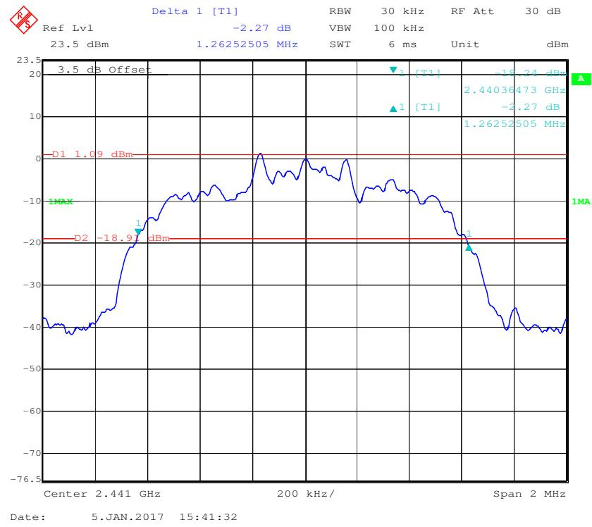
**EDR ( $\pi/4$ -DQPSK): High Channel**
