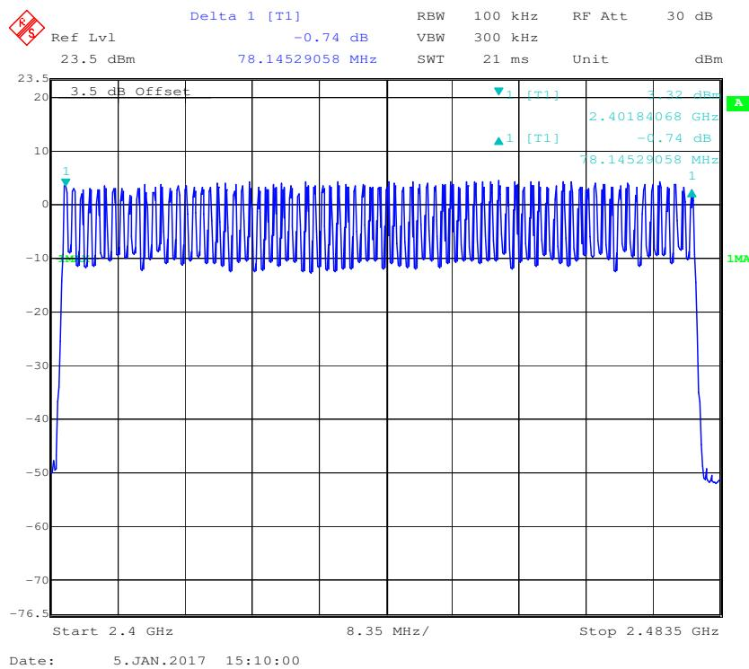
**EDR ( $\pi/4$ -DQPSK): Number of Hopping Channels**
