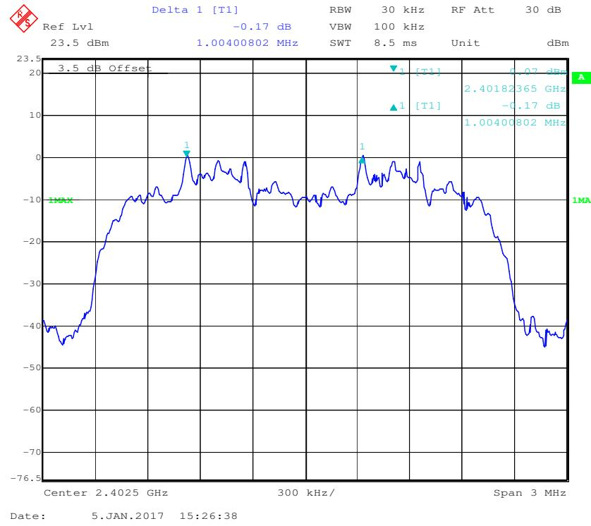
**EDR ( $\pi/4$ -DQPSK): Middle Channel**
