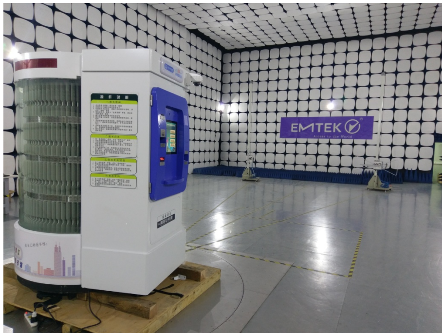
Photo of Radiated Emission Measurement
