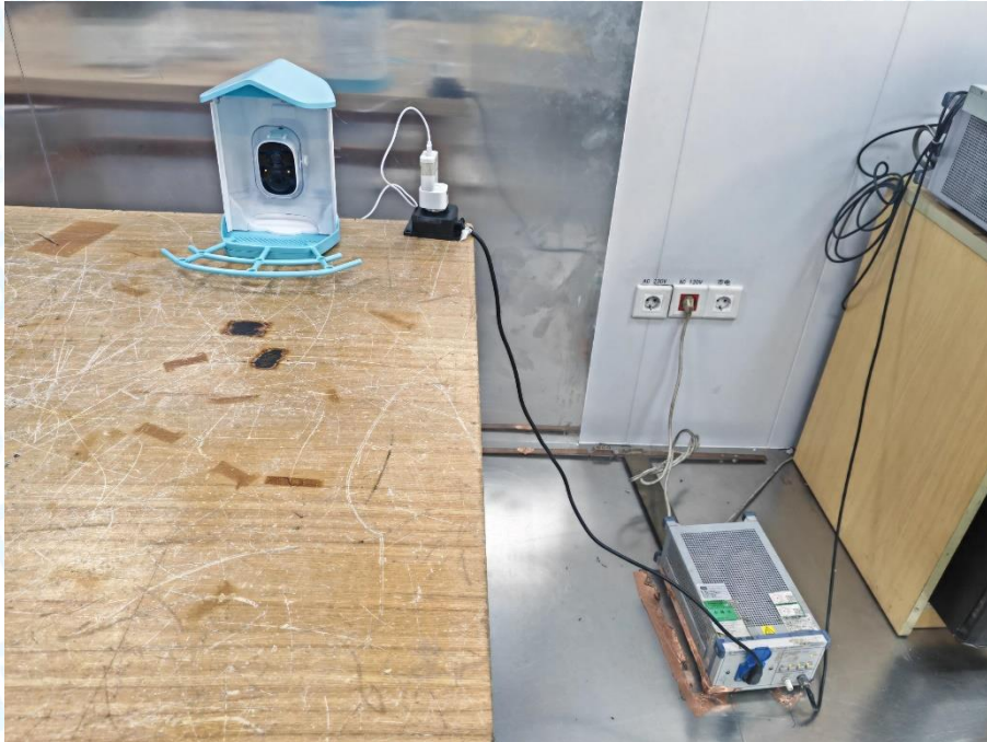
Photo of Setup for Radiated Emission (30MHz~1GHz)
