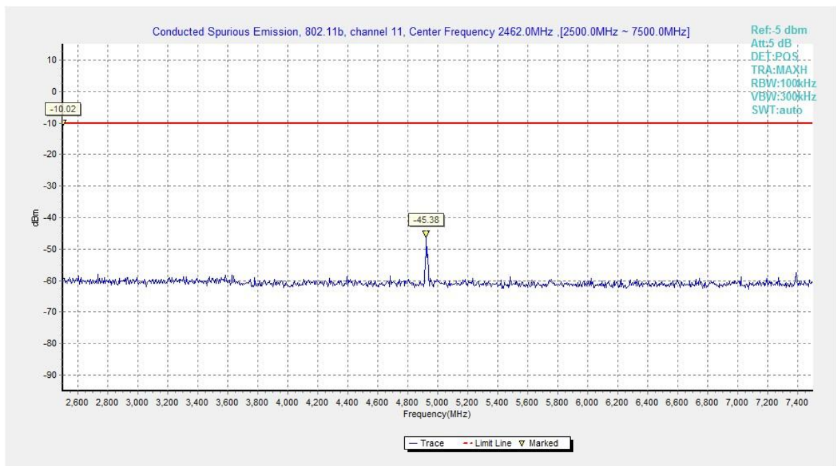
Fig.A.6.1.20 Transmitter Spurious Emission - Conducted (802.11b, Ch11, 2.5 GHz-7.5 GHz)
