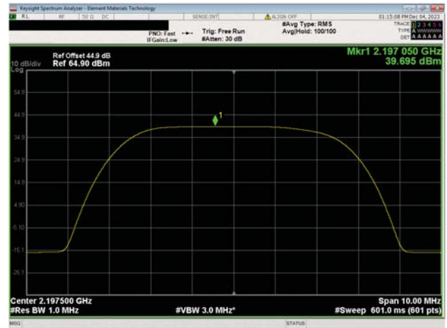
AWS Band n66, 2110 MHz - 2200 MHz 5 MHz Bandwidth 16QAM Modulation High Ch, 2197.5 MHz
