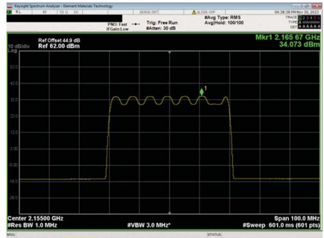
AWS Band n66, 2110 MHz - 2200 MHz 40 MHz Bandwidth 16QAM Modulation Mid Ch, 2155.0 MHz
