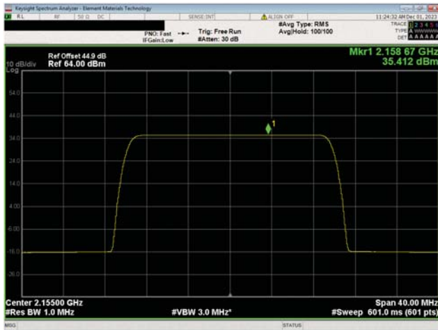
AWS Band n66, 2110 MHz - 2200 MHz 20 MHz Bandwidth QPSK Modulation Mid Ch, 2155.0 MHz
