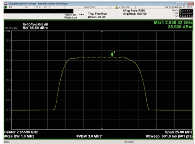
BRS Band n7, 2620 MHz - 2690 MHz 10 MHz Bandwidth 16QAM Modulation Mid Ch, 2655.0 MHz
