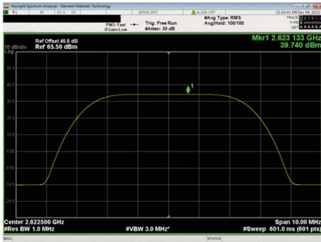
BRS Band n7, 2620 MHz - 2690 MHz 5 MHz Bandwidth QPSK Modulation Low Ch, 2622.5 MHz
