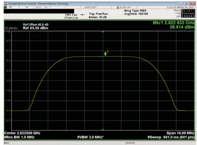
BRS Band n7, 2620 MHz - 2690 MHz 5 MHz Bandwidth 256QAM Modulation Low Ch, 2622.5 MHz
