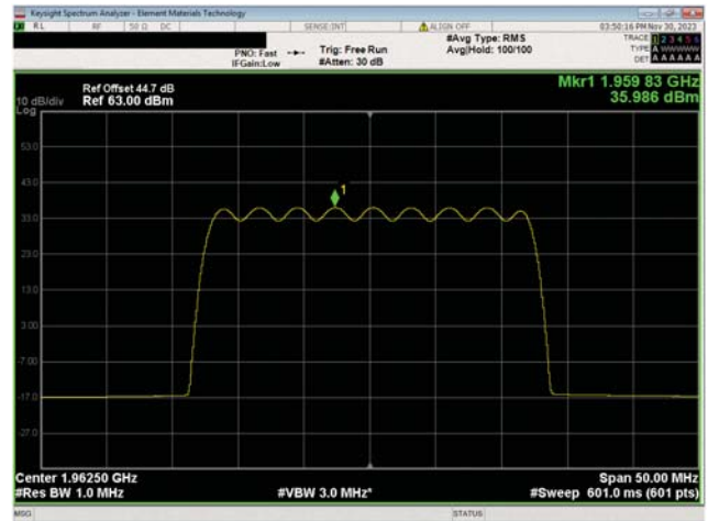
PCS Band n25, 1930 MHz - 1995 MHz 25 MHz Bandwidth 16QAM Modulation Mid Ch, 1962.5 MHz
