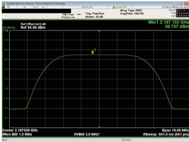
AWS Band n66, 2110 MHz - 2200 MHz 5 MHz Bandwidth 64QAM Modulation High Ch, 2197.5 MHz
