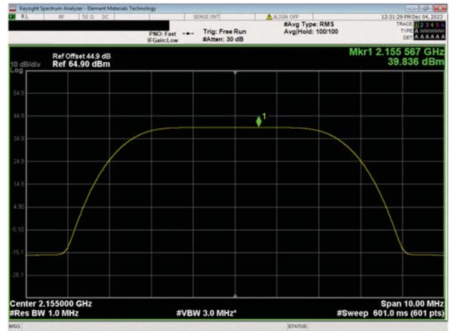
AWS Band n66, 2110 MHz - 2200 MHz 5 MHz Bandwidth QPSK Modulation Mid Ch, 2155.0 MHz
