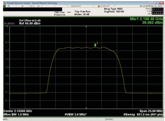
AWS Band n66, 2110 MHz - 2200 MHz 10 MHz Bandwidth 16QAM Modulation Mid Ch, 2155.0 MHz
