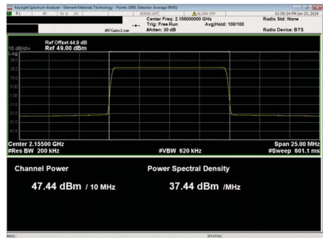
PCS Multicarrier Multiband Test Case 1 QPSK Modulation AWS Band n66, NR10, Mid Ch, 2155.0 MHz
