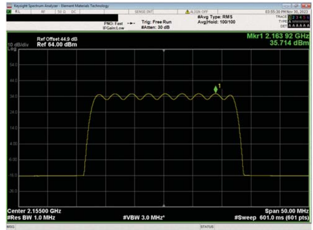
AWS Band n66, 2110 MHz - 2200 MHz 25 MHz Bandwidth 16QAM Modulation Mid Ch, 2155.0 MHz
