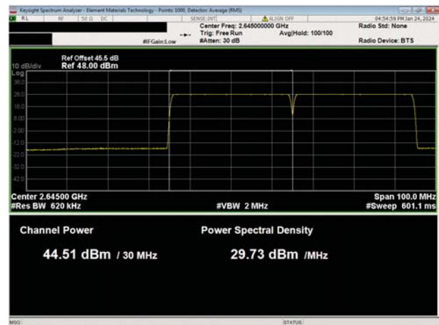
BRS Multicarrier Multiband Test Case 3 QPSK Modulation BRS Band n7, NR30, High Ch, 2645.0 MHz
