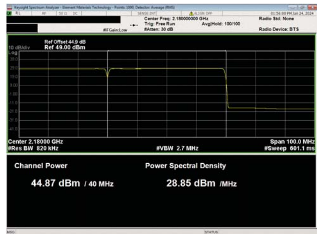
AWS Multicarrier Multiband Test Case 3 QPSK Modulation AWS Band n66, NR40, High Ch, 2180.0 MHz
