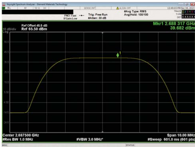
BRS Band n7, 2620 MHz - 2690 MHz 5 MHz Bandwidth QPSK Modulation High Ch, 2687.5 MHz
