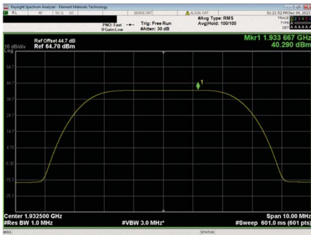
PCS Band n25, 1930 MHz - 1995 MHz 5 MHz Bandwidth 64QAM Modulation Low Ch, 1932.5 MHz
