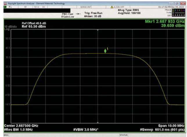
BRS Band n7, 2620 MHz - 2690 MHz 5 MHz Bandwidth 16QAM Modulation High Ch, 2687.5 MHz
