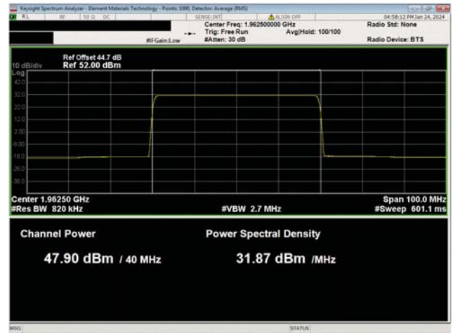
BRS Multicarrier Multiband Test Case 3 QPSK Modulation PSC Band n25, NR40, Mid Ch, 1962.5 MHz
