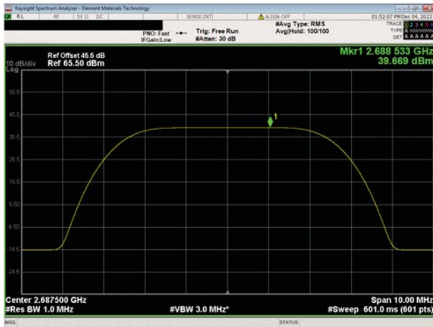
BRS Band n7, 2620 MHz - 2690 MHz 5 MHz Bandwidth 64QAM Modulation High Ch, 2687.5 MHz
