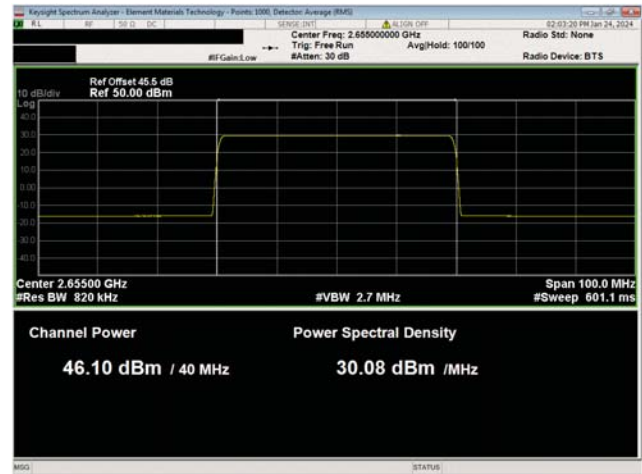
AWS Multicarrier Multiband Test Case 3 QPSK Modulation BRS Band n7, NR40, Mid Ch, 2655.0 MHz
