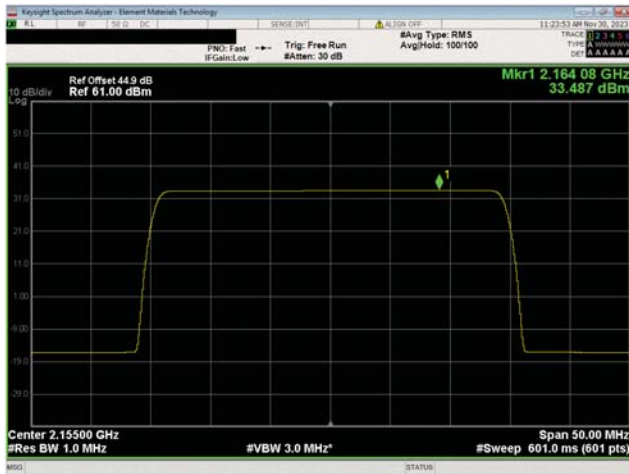
AWS Band n66, 2110 MHz - 2200 MHz 30 MHz Bandwidth QPSK Modulation Mid Ch, 2155.0 MHz
