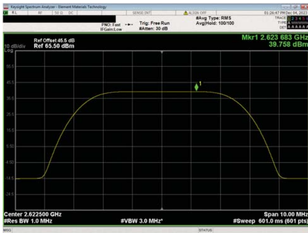
BRS Band n7, 2620 MHz - 2690 MHz 5 MHz Bandwidth 64QAM Modulation Low Ch, 2625.0 MHz
