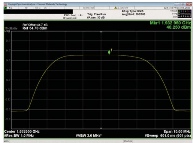
PCS Band n25, 1930 MHz - 1995 MHz 5 MHz Bandwidth 16QAM Modulation Low Ch, 1932.5 MHz
