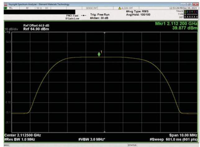
AWS Band n66, 2110 MHz - 2200 MHz 5 MHz Bandwidth 16QAM Modulation Low Ch, 2112.5 MHz
