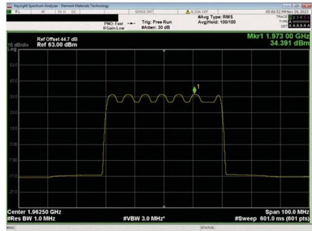
PCS Band n25, 1930 MHz - 1995 MHz 40 MHz Bandwidth 16QAM Modulation Mid Ch, 1962.5 MHz
