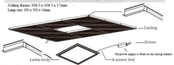
The minimum length of t-shaped protruding supporting lamps is 3.0mm The minimum thickness of t-shaped protruding supporting lamps is 1.0mm
