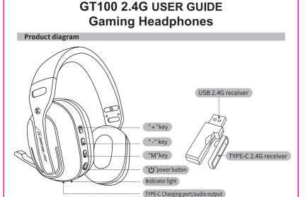
• Power on: 【long press】 "ひ" power button for 3 seconds, after the white and green lights alternately
