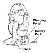
To charge the battery pack, plug it into the transmitter's charging portal. The battery pack automatically begins charging and the CHARGE indicator lights.
