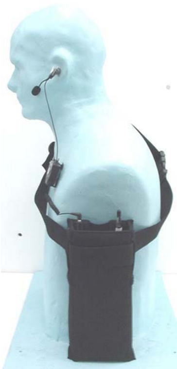
Back Side of DUT facing body - worst-case antenna configuration in relation to left arm
