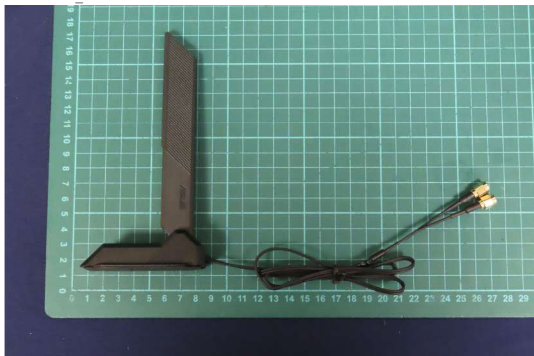
(28) EUT Photo _Wi-Fi & Bluetooth Antenna
