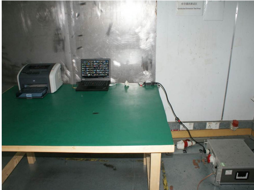
Photograph 6: Set-up for Radiated Emissions, below 1GHz
