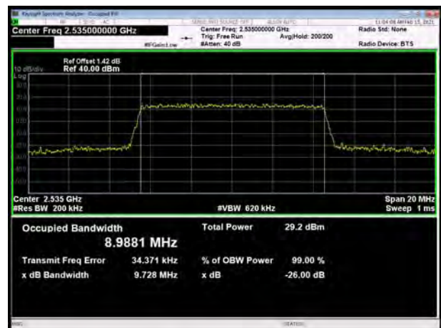
LTE Band 7 64QAM 10MHz CH-High
