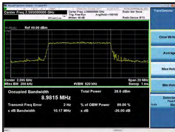
LTE Band 41 16QAM 10MHz CH-High
