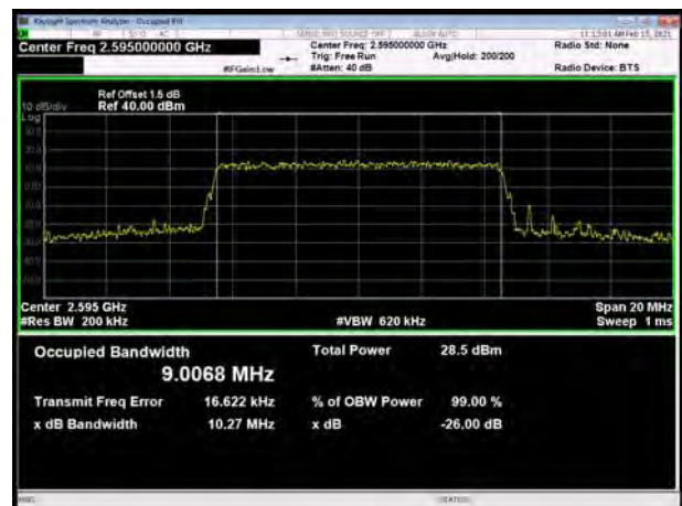
LTE Band 38 64QAM 10MHz CH-High
