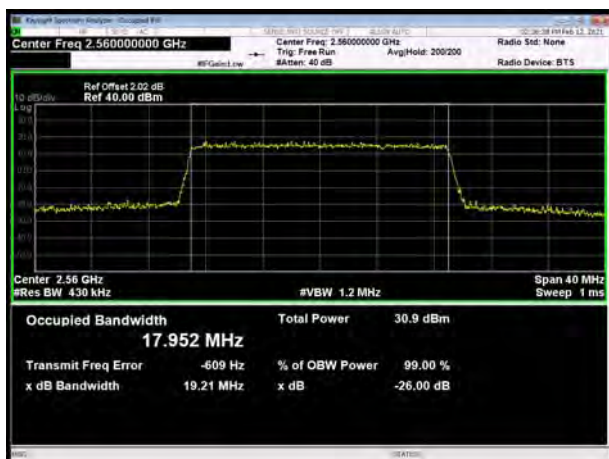
LTE Band 7 QPSK 20MHz CH-High
