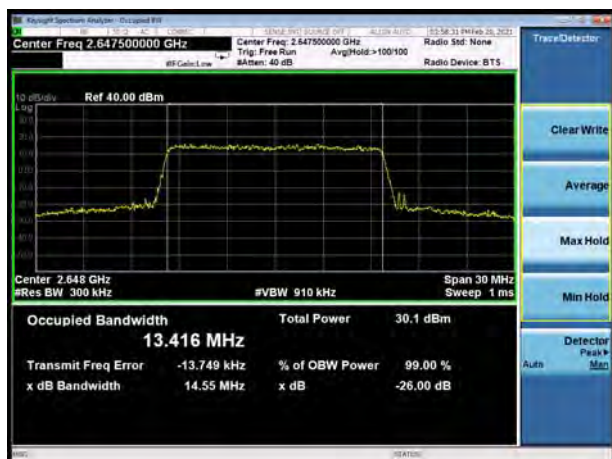
LTE Band 41 QPSK 15MHz CH-High
