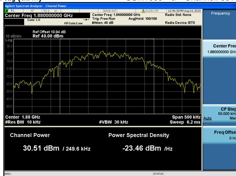
$$\text{PAPR (dB)} = P_{Pk} (\text{dBm}) - P_{Avg} (\text{dBm}) = 30.80 \text{ dBm} - 30.51 \text{ dBm} = 0.29 \text{ dB}$$
