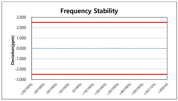
Note. Based on the results of the frequency stability test at the center channel the frequency deviation results measured are very small. As such it is determined that the channels at the band edge would remain inband when the maximum measured frequency deviation noted during the frequency stability tests is applied. Therefore the device is determined to remain operating in band over the temperature and voltage range as tested.
