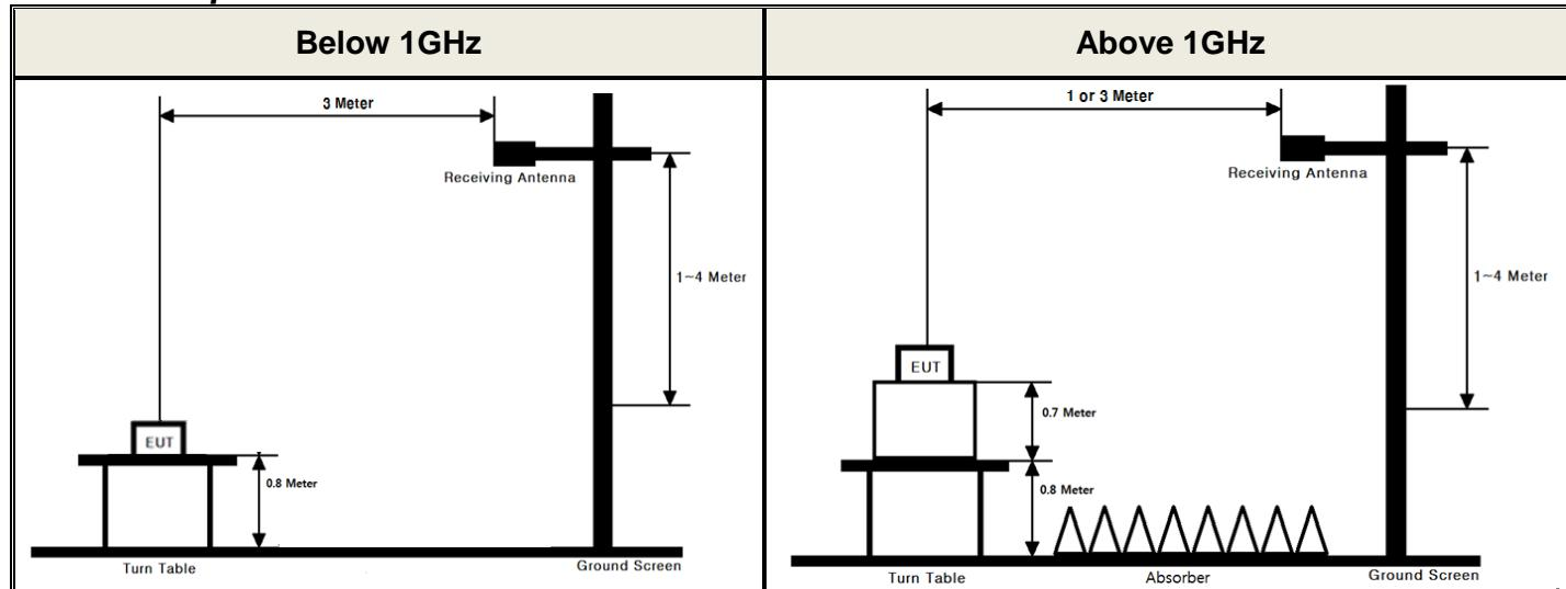
These measurements were performed at 3 m test site. The equipment under test is placed on a non-conductive table 1.5-meters above a turntable which is flush with the ground plane and 3 meters from the receive antenna. For measurements above 1 GHz absorbers are placed on the floor between the turn table and the antenna mast in such a way so as to maximize the reduction of reflections. For measurements below 1 GHz, the absorbers are removed.
