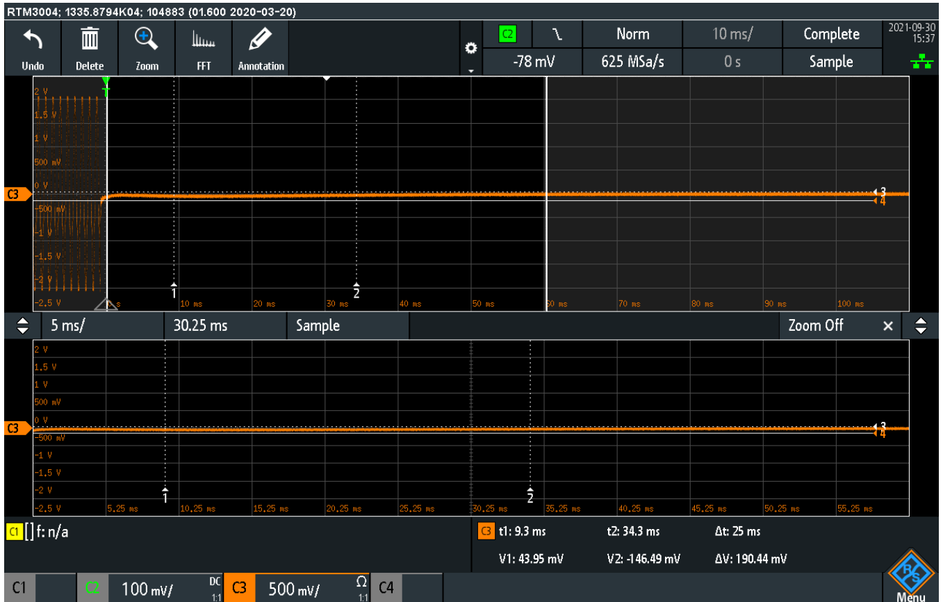
Plot 7.6.5 Transient frequency during power ON test results at mid carrier frequency
