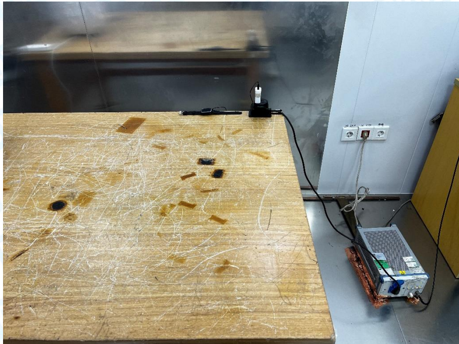
Photo of Setup for Radiated Emission (30MHz~1GHz)
