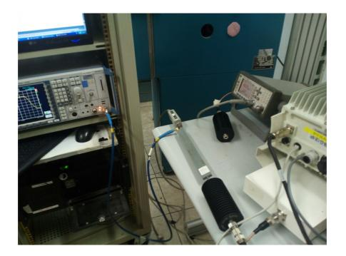
Photograph No.2 Conducted spurious emissions, occupied bandwidth measurement setup
