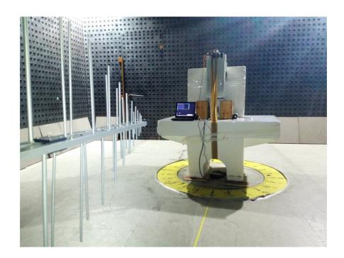
$\label{eq:Photograph No.6} Photograph No.6 Spurious emissions measurement setup in the anechoic chamber in 1 – 18 GHz$
