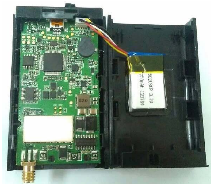
Figure 5. Backup Battery Installation
