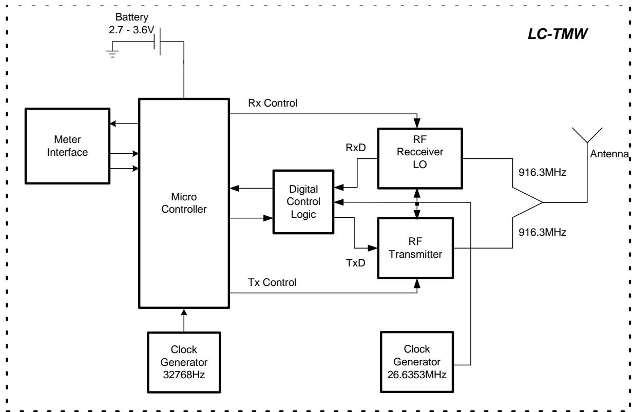
Figure 1: LC-TMW Block Diagram
