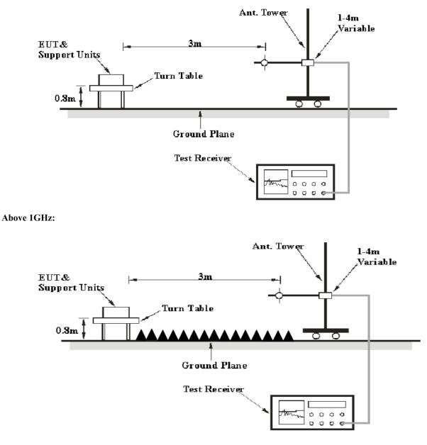
The radiated emission tests were performed in the 3 meters chamber test site, using the setup accordance with the ANSI C63.4-2014. The specification used was the FCC Part 15.109 limits.
