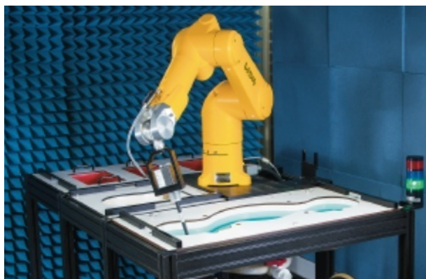
Fig 6.5 Photo of DASY5
