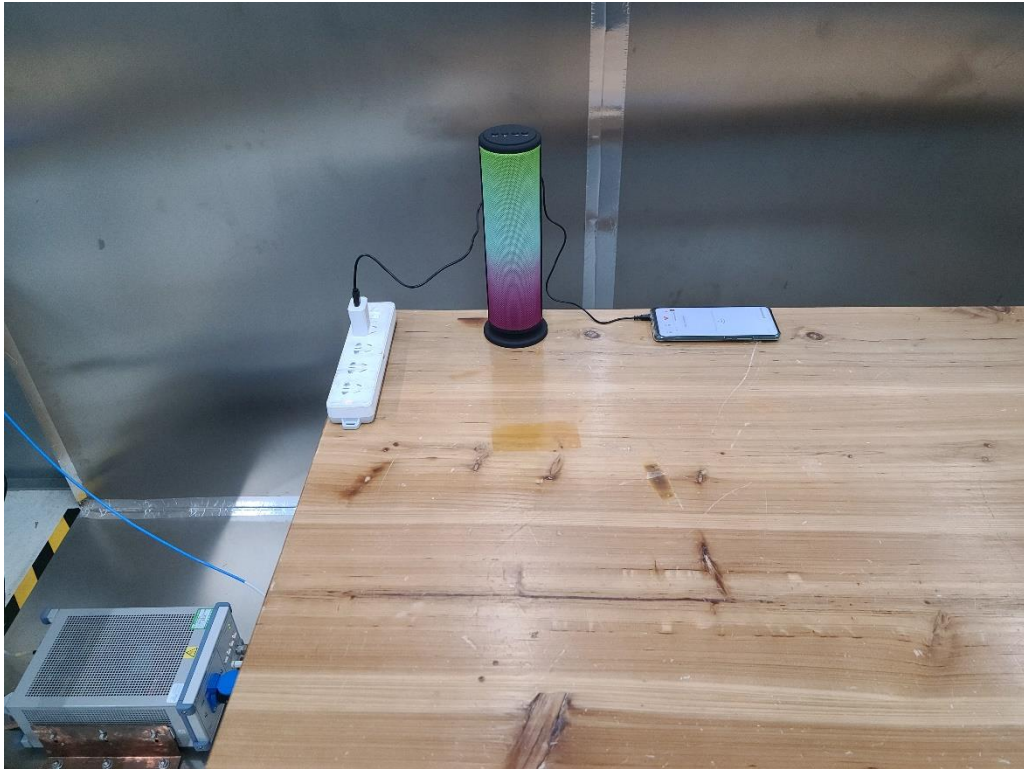
Photograph 2: Set-up for Radiated Emissions, below 1GHz
