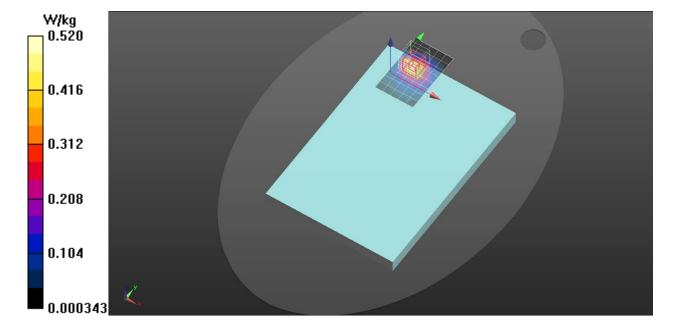
Frequency: 2610 MHz; Duty Cycle: 1:1; Room Ambient Temperature: 23.0°C; Liquid
