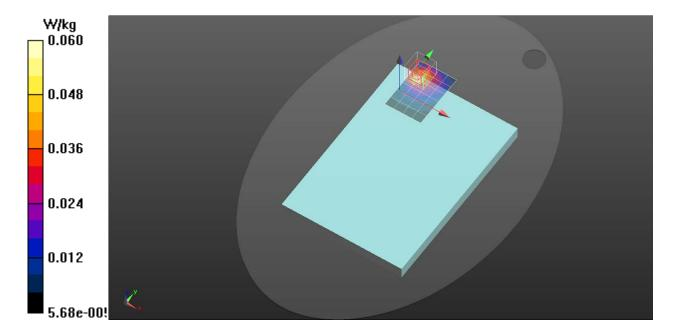
Frequency: 1850 MHz; Duty Cycle: 1:1; Room Ambient Temperature: 23.0°C; Liquid
