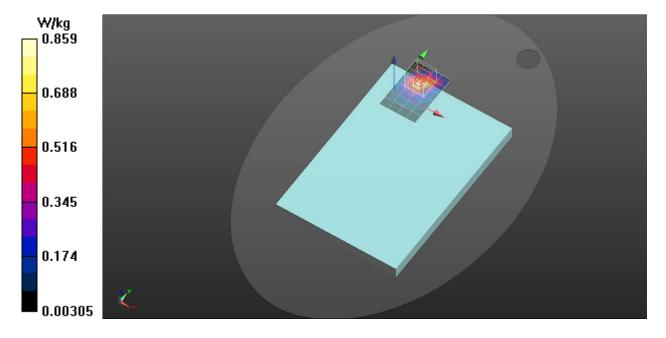
Frequency: 673 MHz; Duty Cycle: 1:1; Room Ambient Temperature: 23.0°C; Liquid
