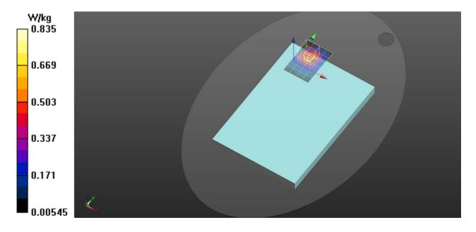
Frequency: 1745 MHz; Duty Cycle: 1:1; Room Ambient Temperature: 23.0°C; Liquid
