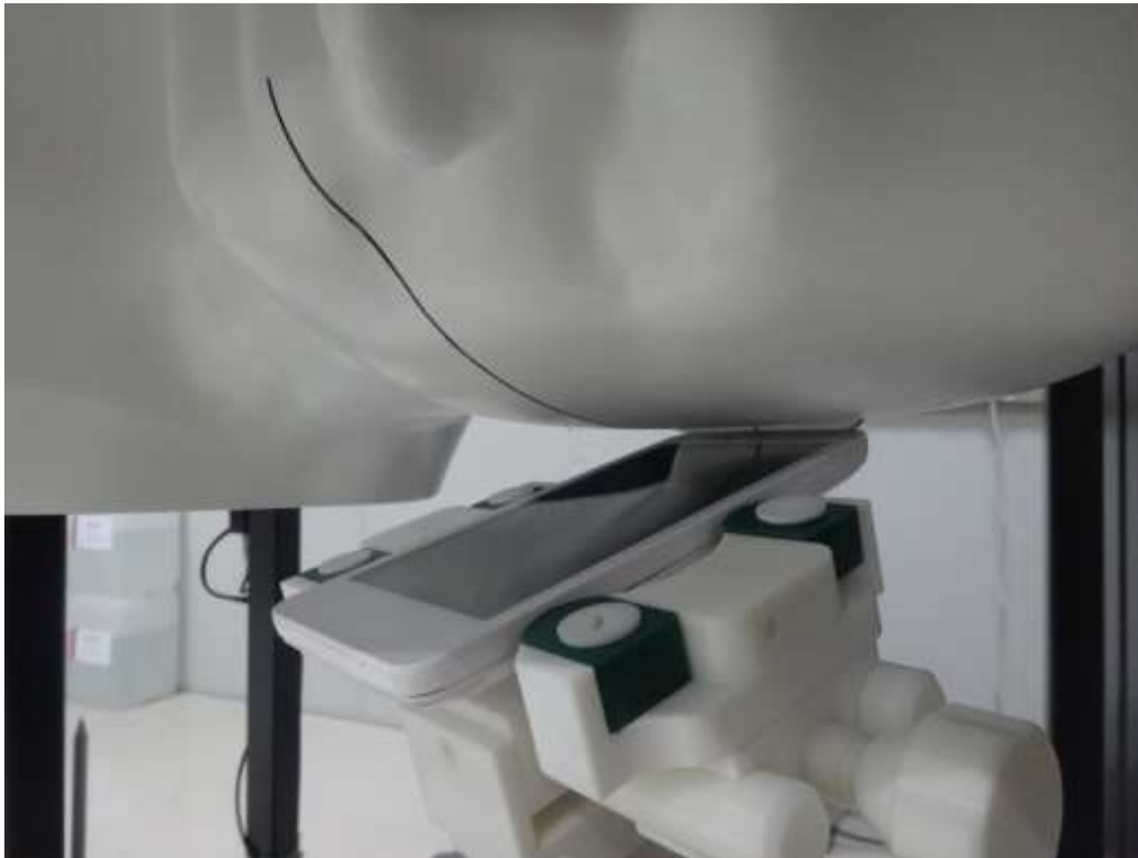
Head Setup Photo(Left Tilt )
