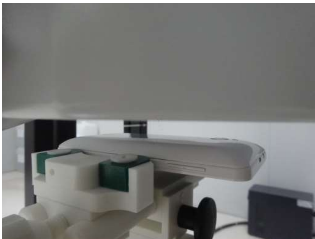
15mm body-worn Back Side Setup Photo
