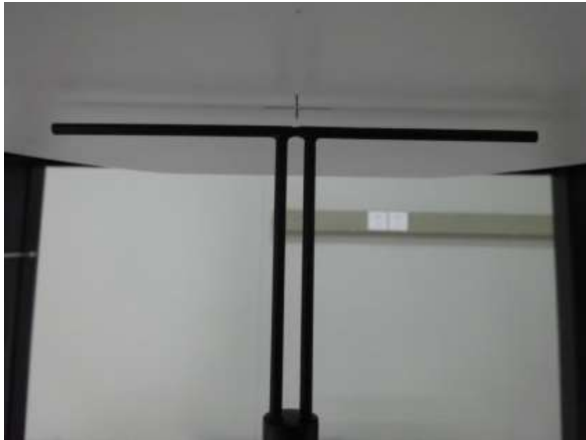
Photo of Dipole Setup
