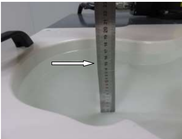
Pictures for Head and Body Liquid 2450MHz(DEPTH>15cm)
