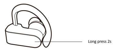
Methold 2: Press MFB for 2s to power on( LED light turn on green
