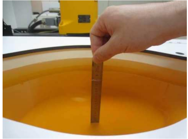
Liquid Depth in the flat phantom(18.2cm)
