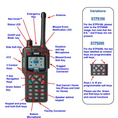
Sepura plc Radio House, St Andrew's Road, Cambridge, CB4 1GR England www.sepura.com Switching On Press and release the Mode Key.
