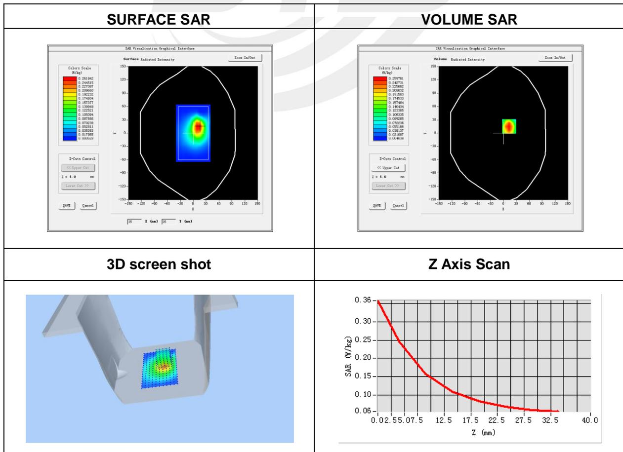
**Plot 2: DUT: GPS Tracker; EUT Model: TRKM015-LC**
