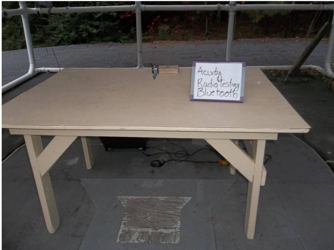
**Figure 6. Intentional Radiated Emission Test Setup, Front**
