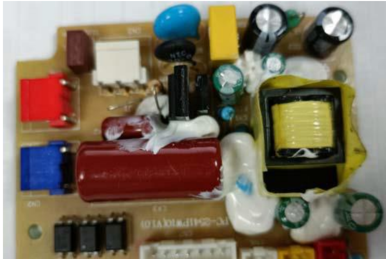
New Switching power board
