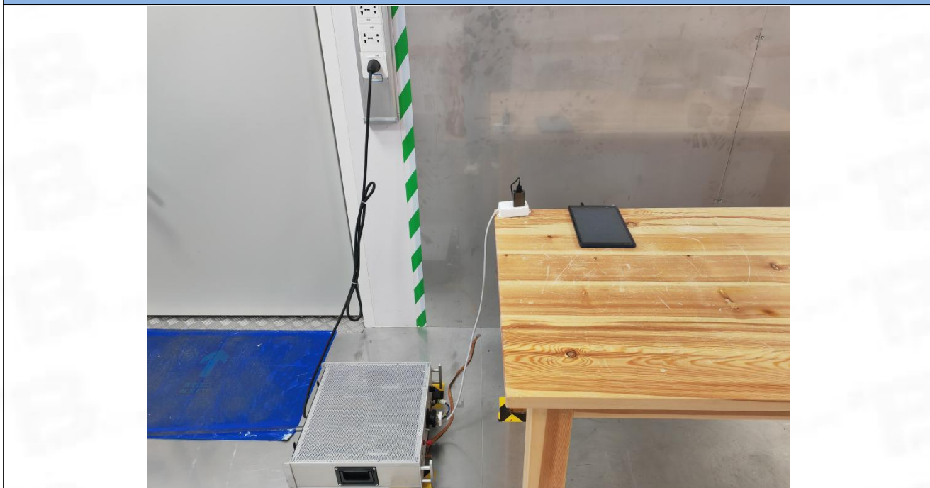
Conducted Emission at AC power line
