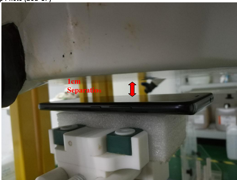
Body Setup Photo (LCD UP)
