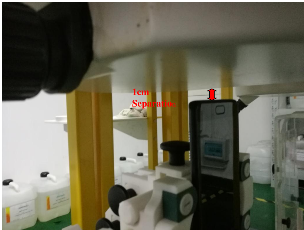
Body Setup Photo (BOTTOM EDGE)
