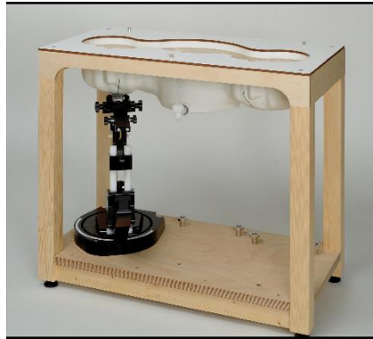
Picture C.10: SAM Twin Phantom
