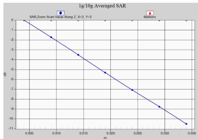
Fig.A.1- 11 Z-Scan at power reference point (LTE Band2)
