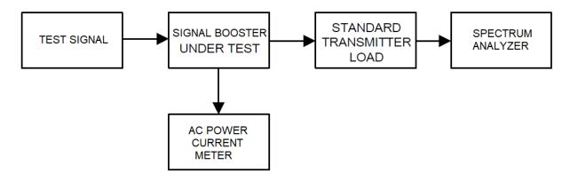
Test Data: Power to Final Amplifier Calculation
