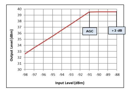
Max Power Output at Saturation: 39.56 dBm
