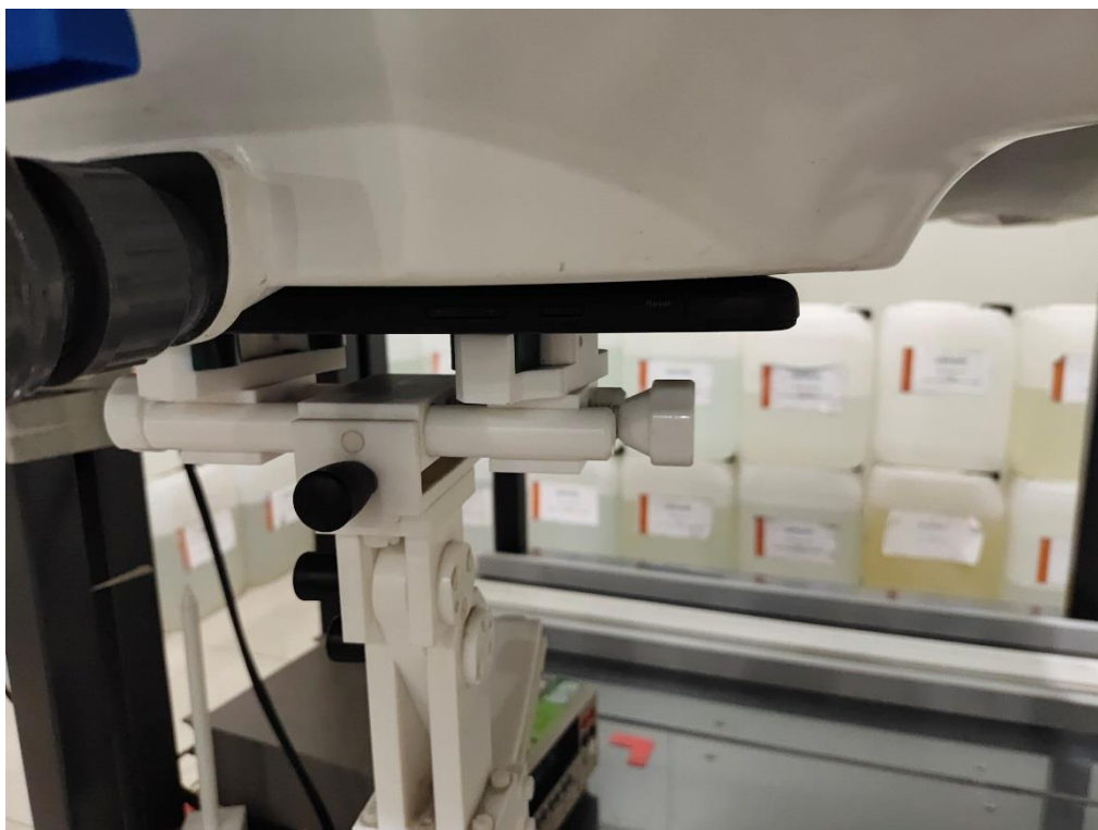
Body Back side(separation distance is 0mm)
