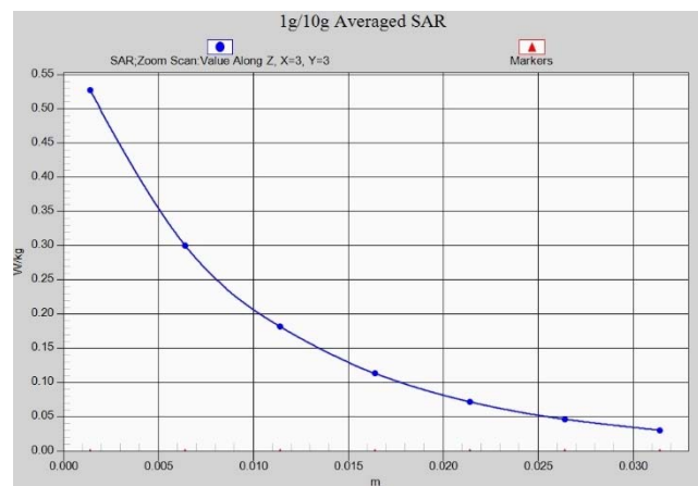
Fig. 1-14 Z-Scan at power reference point (LTE Band2)
