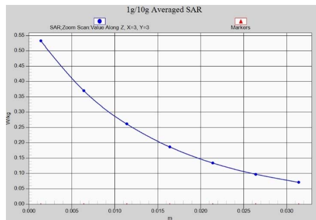
Fig. 1-23 Z-Scan at power reference point (LTE Band12)
