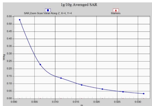
Fig. 1-15 Z-Scan at power reference point (LTE Band2)
