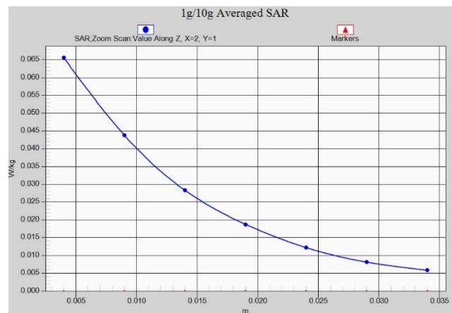
Fig. 1-4 Z-Scan at power reference point (1900 MHz)
