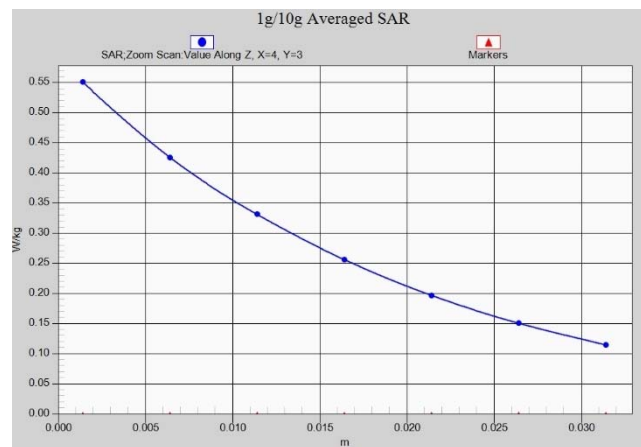
Fig. 1-16 Z-Scan at power reference point (LTE Band2)
