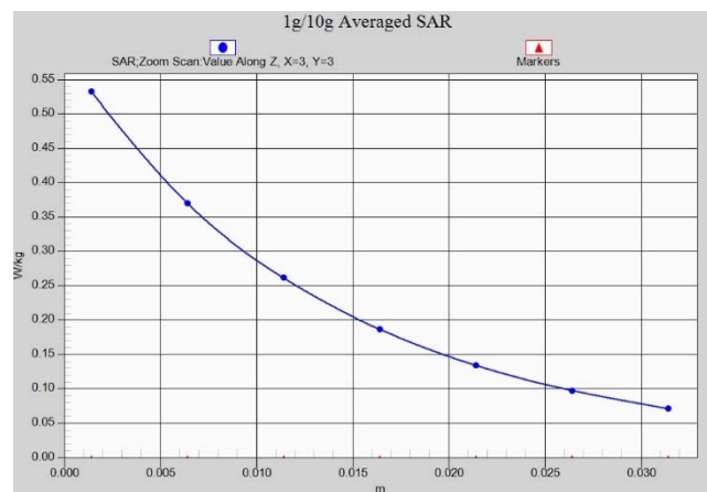
Fig. 1-18 Z-Scan at power reference point (LTE Band5)
