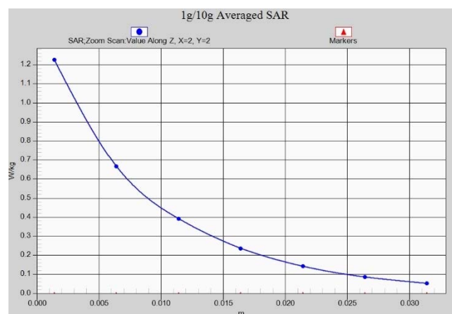
Fig. 1-5 Z-Scan at power reference point (1900 MHz)
