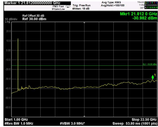
Channel: BOTTOM, Modulation: QPSK, BW=15MHz, Range: Upper
