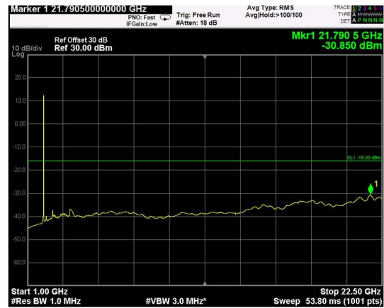
Channel: BOTTOM, Modulation: 16QAM, BW=15MHz, Range: Upper
