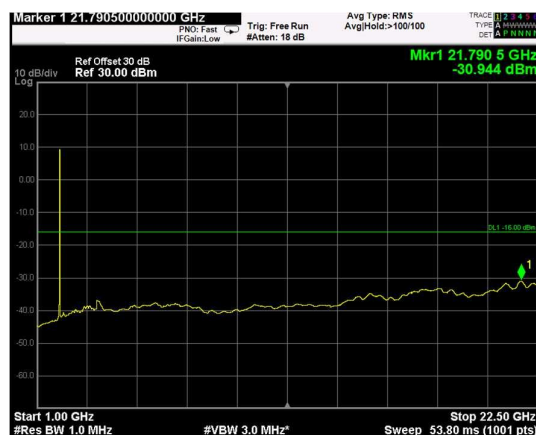
Channel: TOP, Modulation: QPSK, BW=5MHz, Range: Upper
