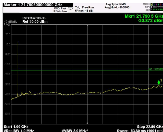
Channel: TOP, Modulation: 64QAM, BW=20MHz, Range: Upper
