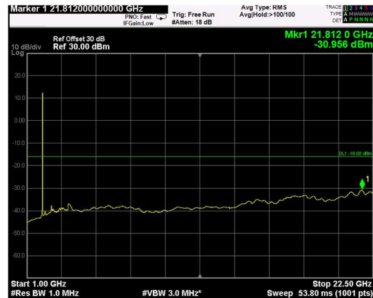
Channel: MIDDLE, Modulation: 16QAM, BW=20MHz, Range: Upper
