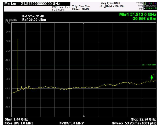
Channel: MIDDLE, Modulation: 256QAM, BW=15MHz, Range: Upper
