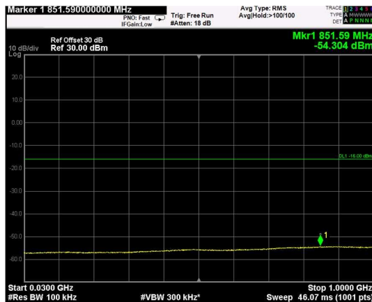
Channel: BOTTOM, Modulation: QPSK, BW=5MHz, Range: Lower
