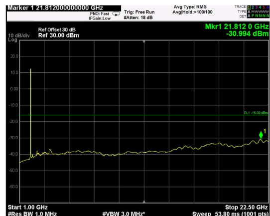
Channel: TOP, Modulation: 256QAM, BW=15MHz, Range: Upper
