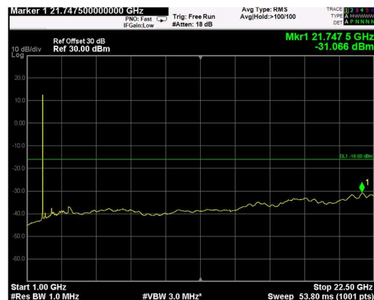
Channel: TOP, Modulation: 16QAM, BW=15MHz, Range: Upper
