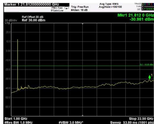
Channel: TOP, Modulation: 16QAM, BW=20MHz, Range: Upper
