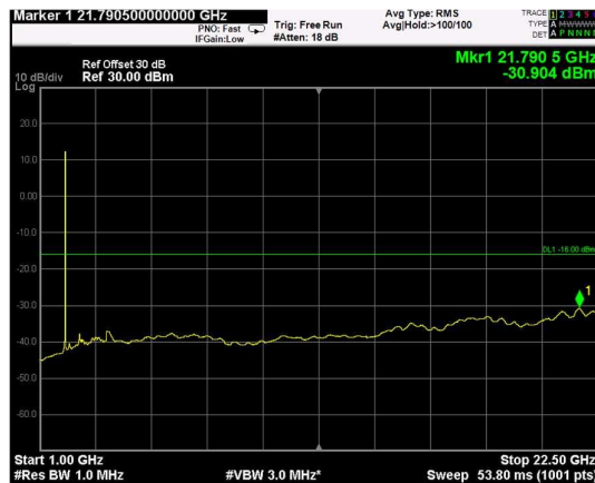
Channel: MIDDLE, Modulation: QPSK, BW=20MHz, Range: Upper
