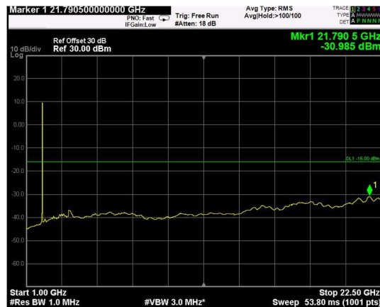
Channel: BOTTOM, Modulation: QPSK, BW=5MHz, Range: Upper
