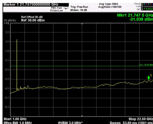
Channel: TOP, Modulation: 256QAM, BW=10MHz, Range: Upper
