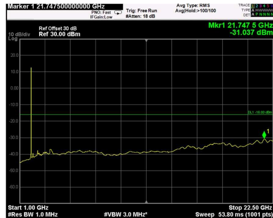
Channel: MIDDLE, Modulation: 16QAM, BW=15MHz, Range: Upper
