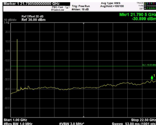
Channel: MIDDLE, Modulation: 64QAM, BW=20MHz, Range: Upper
