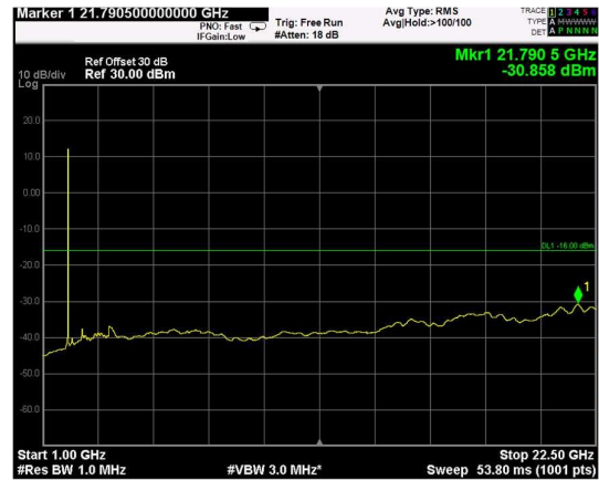
Channel: MIDDLE, Modulation: QPSK, BW=15MHz, Range: Upper
