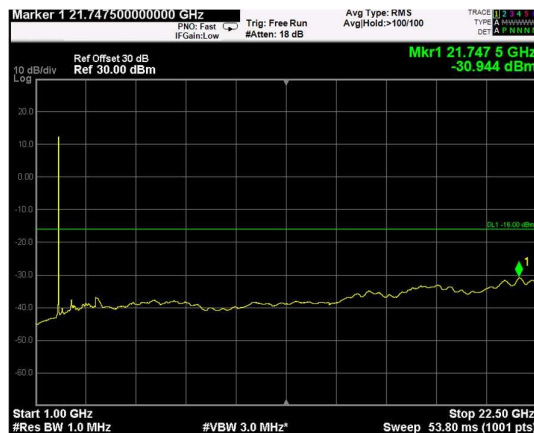
Channel: BOTTOM, Modulation: 64QAM, BW=15MHz, Range: Upper
