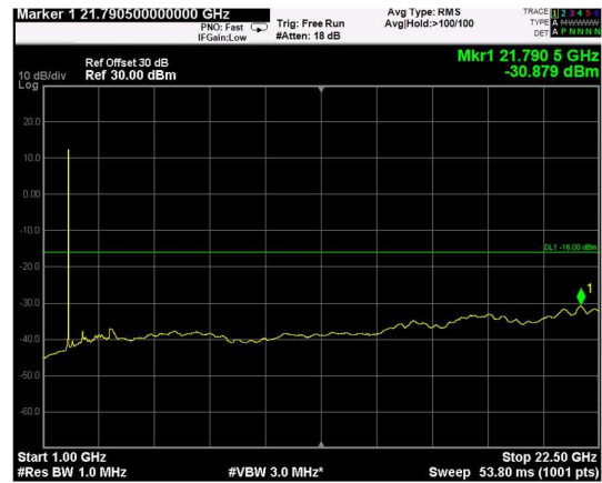
Channel: BOTTOM, Modulation: 256QAM, BW=20MHz, Range: Upper
