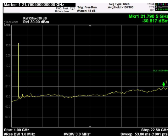
Channel: BOTTOM, Modulation: 256QAM, BW=10MHz, Range: Upper
