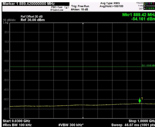
Channel: MIDDLE, Modulation: 16QAM, BW=5MHz, Range: Lower
