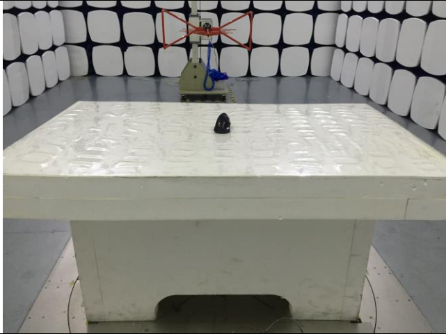
Radiated Spurious Emissions Test Setup Below 1GHz
