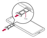
5 Firmly push the tray into the end and make sure that there are no gaps between the terminal and the cover (P.38).
