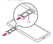
Push the tray into the end, firmly press each point indicated with O, and then make sure that there are no gaps between the terminal and the cover.
