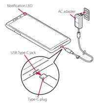
When charging is complete, remove the power plug of the AC adapter from the power outlet, and then remove the Type-C plug horizontally from the terminal.
