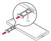
5 Firmly push the tray into the end and make sure that there are no gaps between the terminal and the cover (P.35).
