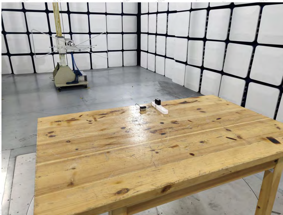
Photo of Radiation Emission Test
