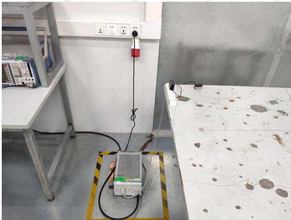
Photo of Conducted Emission Measurement
