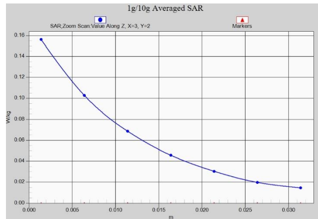
Fig. 3-1 Z-Scan at power reference point (1900 MHz)
